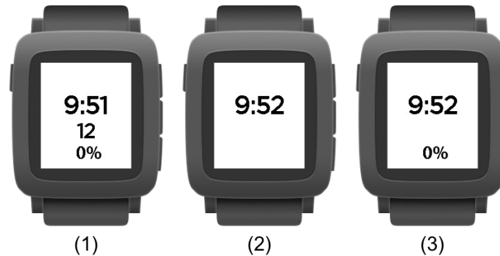
Fig. 2. Smartwatch displays when the button is pressed. (1) Visual Only: displays step count value and percentage towards the goal. (2) Tactile Only: the screen does not change and the last encoded vibrations are re-played. (3) Hybrid: Visual/Tactile: displays percentage achieved towards the goal.
