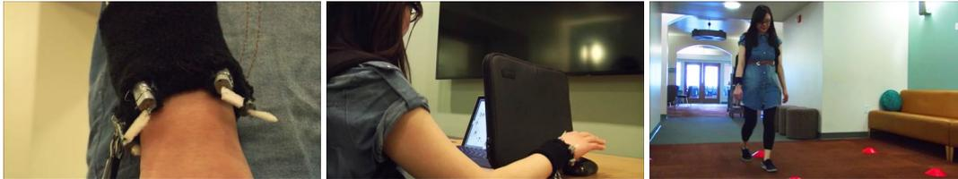
Figure 1. Left to right: A user wearing a novel haptic wearable prototype, comparing the recognizability of haptic cues with different forms of tactile stimulation, following navigational instructions through haptic cues.
